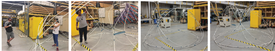
Figure 6. Installation of tensile struts to resist dead loads.
