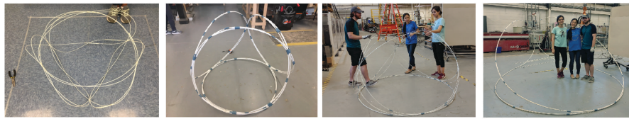
Figure 5. Figure 5. (L-R) 5A: 1/6 scale model (left); 5B: 1/4 scale model from 2 No.1/4" diam. rods; 5C: 1/4 scale model from 2 No.3/16" diam. rods; and 5D: full-scale 'pringle' model (right).
