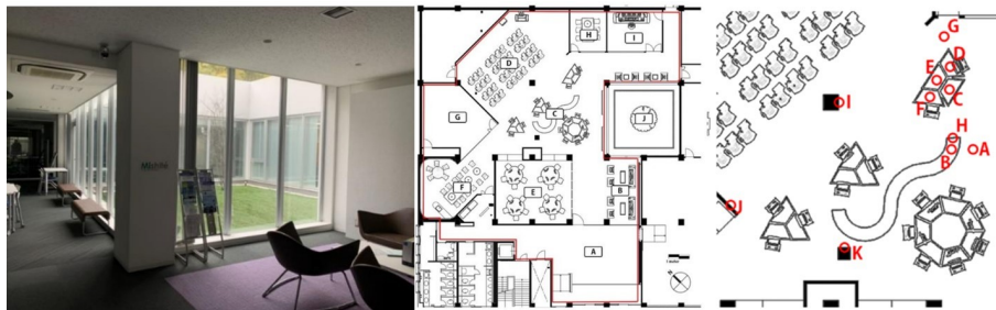
Figure 3. (left) the lounge area in the selected case study. (middle) different functional areas within the selected case study, the measurement points included in the study are in areas C and D, J represents the courtyard. (Right) Sensor points selected for comparison, points H, I, J, and K are on vertical surfaces.
